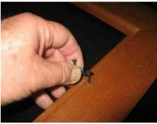
**Step 5** - Remove tape and align screw with pilot hole.
