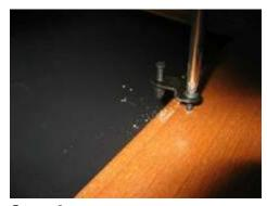
**Step 6** - Screw down with hand screwdriver only until you can barely swing the metal clip.
