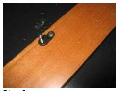
**Step 8** - All metal clips should be swung over like this giving full clearance for the glass.
