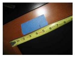
**Step 1** - From the back of the frame measure from the bottom up on the left & right sides 5 inches and make a mark. Repeat from the top down. You should have 4 marks.
